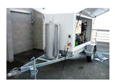
Vacuum System with high capacity vacuum pump & blower set for pulling vacuum on transformer main tanks prior to filling. Can be a separate unit, or combined with the Trojan HVP with total capacity designed to suit.
